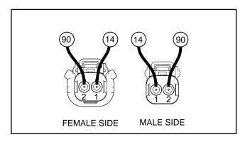
Figure 25. C3 Choke Solenoid Connector
